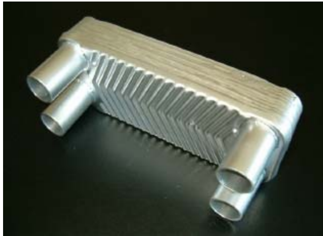
Figure 14 CatHex reactor for PROX. The reactor consists of catalytically active plates which are assembled into a plate-type heat exchanger. Volume \approx 0.5 litre/kW e .
