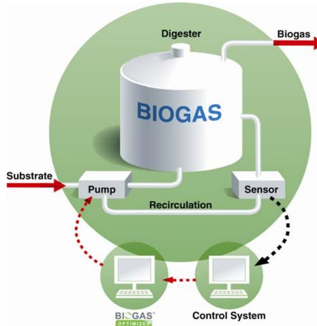
Biogas Optimizer™ provides biogas producers with a system for on-line monitoring and intelligent supervisory control of biogas digesters. The system has the ability to protect a biogas production process from overload, while allowing the maximum utilisation of digester capacity.
