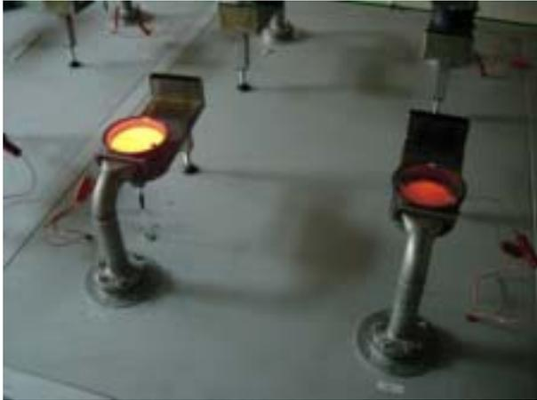
**Figure 1.** Cordierite catalyst (left) vs. Catator wire mesh catalyst (right).
